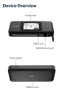
Note: The 1Gbps Ethernet port is disabled by default to extend battery life. To enable it, select Enable Ethernet Port from Menu > Settings on the touchscreen, or Settings > Preferences on the Admin web UI.
