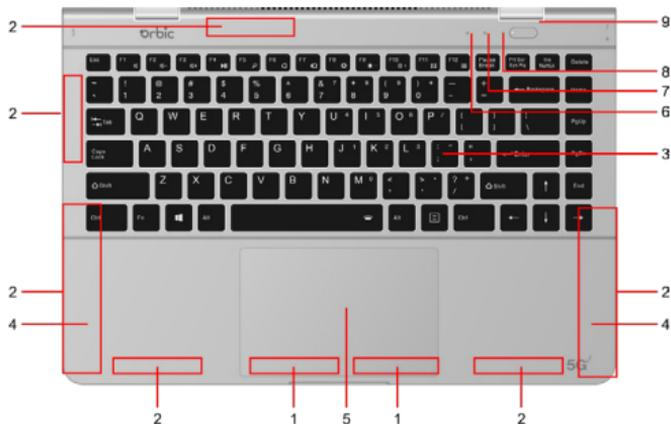
1. **Wi-Fi Antennas:** Send and receive radio waves for the Bluetooth and Wi-Fi modules.
