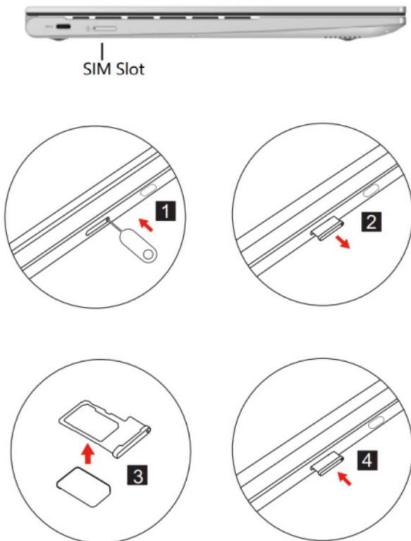
**Step 1.** Use the ejector tool (included) to eject the nano SIM card tray, and then slide the tray out of the computer. If a nano SIM card is installed, gently take the nano SIM card out of the tray.
