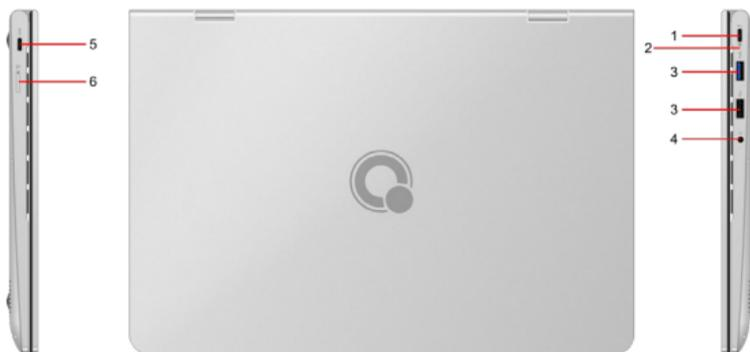
1. **Power Connector/USB-C Connector:** Connect to power with the included power cord and AC power adapter. Connect to an external display, storage, or data device.
