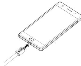
**WARNING:** Use only an approved charging accessory to charge your phone. Improper handling of the charging port, as well as the use of an incompatible charger may cause damage to your device and void the warranty.
